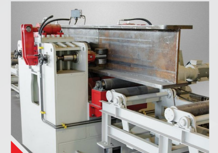
Nắn dầm | Straightening beams
